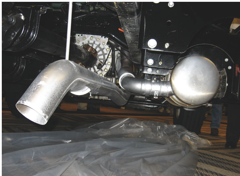
Cat's C7, displayed in a Ford F-650 at an industry meeting, is more tricky to package because its CGI piping emerges from the diesel particulate filter (at right, looking like a muffler) and runs back to the engine.
